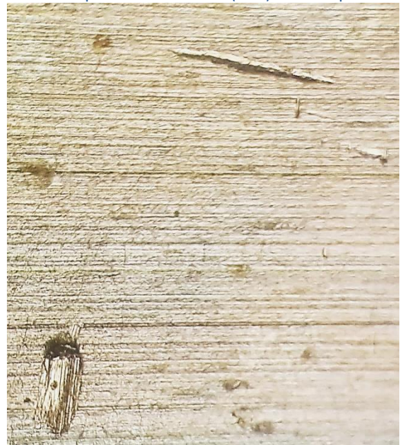
Metallic particles inclusion (40X). Unacceptable
